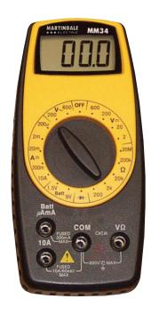
This low cost multimeter has 4 main functions together with diode and battery test and a large clear display.
